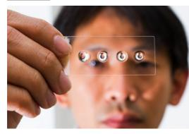
The development of a tiny slipcover lens could lead to the first smartphone microscope, potentially changing the face of disease diagnosis in the developing world.
